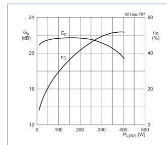
$V_{\rm DS}$  = 50 V;  $I_{\rm Dq}$  = 1.3 A; measured in a common source narrowband 860 MHz test circuit.
