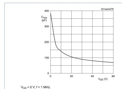
Fig 1. Output capacitance as a function of drain-source voltage; typical values per section
