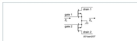
Fig 4. Definition of transistor impedance
