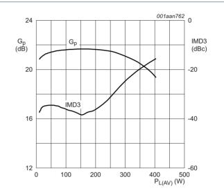
$V_{DS}$  = 50 V;  $I_{Dq}$  = 1.3 A; measured in a common source narrowband 860 MHz test circuit.
