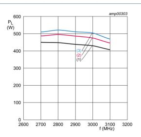
$V_{DS}$  = 32 V;  $I_{Dq}$  = 400 mA;  $t_p$  = 300  $\mu s;$   $\delta$  = 10 %.
