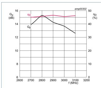
$V_{DS}$  = 32 V;  $I_{Dq}$  = 400 mA;  $P_L$  = 425 W;  $t_p$  = 300  $\mu s;$   $\delta$  = 10 %.
