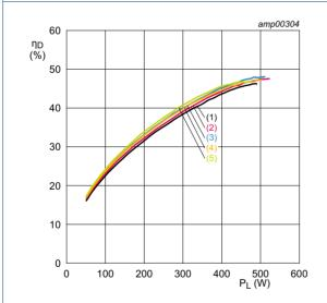
$V_{DS}$  = 32 V;  $I_{Dq}$  = 400 mA;  $t_p$  = 300  $\mu$ s;  $\delta$  = 10 %.
