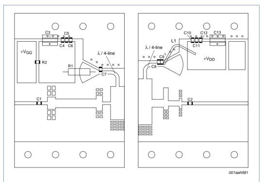
Striplines are on a double copper-clad Rogers Duroid 6006 Printed-Circuit Board (PCB) with  $\epsilon_r$  = 6.2 and thickness = 0.64 mm.
