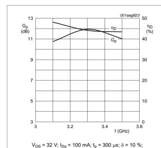
Fig 2. Power gain and drain efficiency as functions of frequency; typical values
