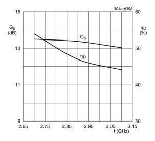
$P_L$  = 120 W;  $V_{DS}$  = 32 V;  $I_{Dq}$  = 100 mA;  $t_p$  = 100  $\mu s$ ;  $\delta$  = 20 %.
