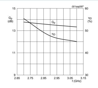
$P_L$  = 120 W;  $V_{DS}$  = 32 V;  $I_{Dq}$  = 100 mA;  $t_p$  = 300  $\mu s$ ;  $\delta$  = 10 %.
