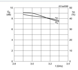
$V_{DS}$  = 32 V;  $I_{Dq}$  = 20 mA;  $t_p$  = 200  $\mu s; \, \delta$  = 12 %;  $P_1 = 100 W.$
