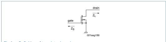
Fig 6. Definition of transistor impedance
