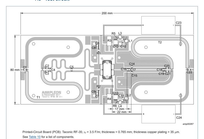
Fig 4. Component layout for class-AB production test circuit
