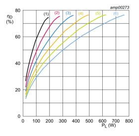
$I_{Dq}$  = 100 mA; f = 108 MHz;  $t_p$  = 100  $\mu$ s;  $\delta$  = 20 %.
