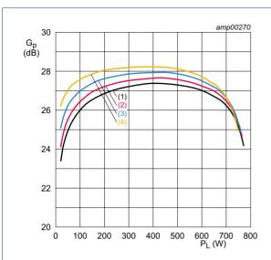
$V_{DS}$  = 50 V; f = 108 MHz;  $t_p$  = 100  $\mu$ s;  $\delta$  = 20 %.
