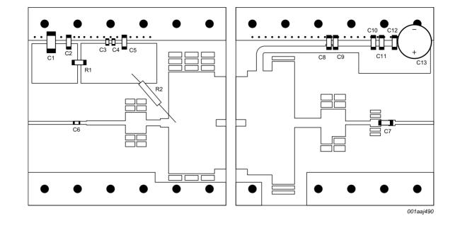
Printed-Circuit Board (PCB): Duroid 6006;  $\varepsilon_r$  = 6.15 F/m; thickness = 0.64 mm; thickness copper plating = 35  $\mu$ m. See Table 9 for a list of components.
