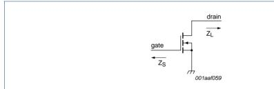
Fig 1. Definition of transistor impedance
