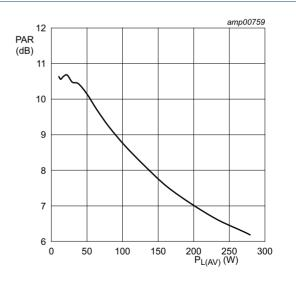
$V_{DS}$  = 50 V;  $I_{Dq}$  = 2 × 650 mA; f = 700 MHz.
