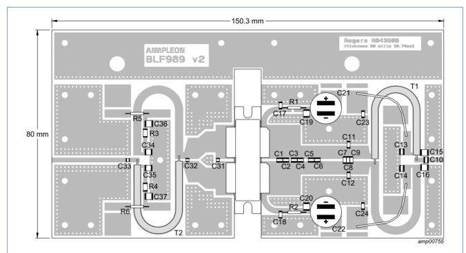
Printed-Circuit Board (PCB): RO4350B:  $\epsilon_r$  = 3.48 F/m; height = 0.762 mm; Cu (top/bottom metallization); thickness copper plating = 35  $\mu$ m. See Table 9 for a list of components.
