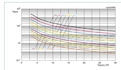
TTF (0.1 % failure fraction).
