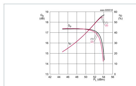
$V_{DS}$  = 28 V;  $I_{Dq}$  = 1740 mA.
