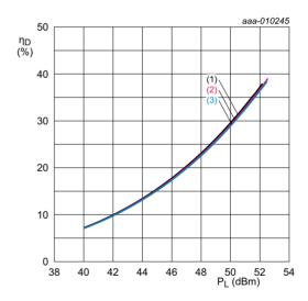
$V_{DS} = 28 \text{ V}; I_{Dq} = 3400 \text{ mA}.$
