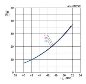
$V_{DS}$  = 28 V;  $I_{Dq}$  = 3400 mA.
