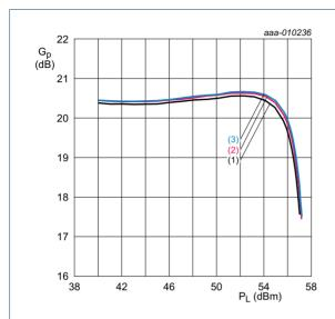
$V_{DS}$  = 28 V;  $I_{Dq}$  = 3400 mA;  $t_p$  = 100  $\mu s; \, \delta$  = 10 %.
