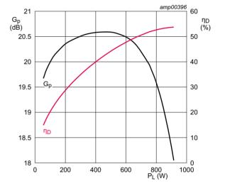
$V_{DS}$  = 50 V;  $I_{Dq}$  = 2 x 900 mA;  $t_p$  = 100  $\mu$ s;  $\delta$  = 10 %.
