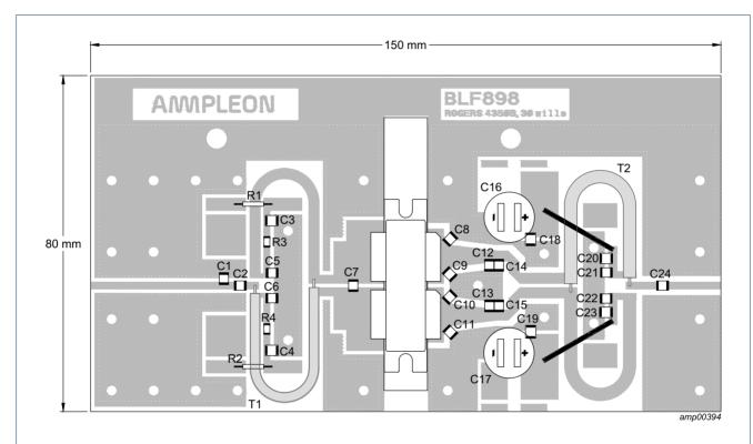
Printed-Circuit Board (PCB): Rogers 4350B:  $\epsilon_r$  = 3.66 F/m, height = 0.762 mm; Cu (top/bottom metalization); thickness copper plating = 35  $\mu$ m. See Table 9 for a list of components.
