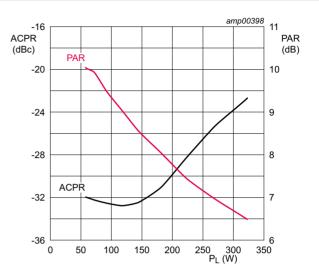
$V_{DS}$  = 50 V;  $I_{Dq}$  = 2 x 900 mA; PAR (of output signal) at 0.01 % probability on CDDF; PAR of input signal = 9.5 dB at 0.01 % probability on CDDF.
