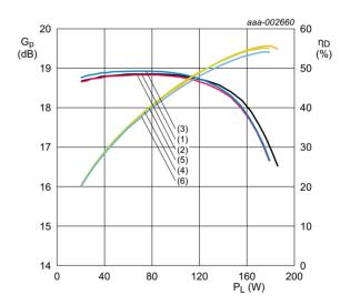
$V_{DS}$  = 28 V;  $I_{Dq}$  = 1200 mA;  $\delta$  = 10 %;  $t_p$  = 0.10 ms.
