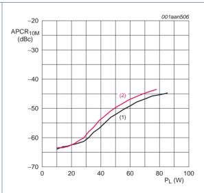
$V_{DS} = 28 \text{ V}; I_{Da} = 900 \text{ mA}.$
