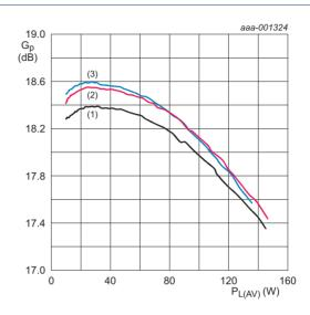
$V_{DS}$  = 28 V;  $I_{Dq}$  = 1900 mA; Channel Spacing = 5 MHz; PAR = 8.4 dB at 0.01 % probability on the CCDF.
