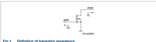
Fig 1. **Definition of transistor impedance**
