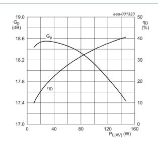
$V_{DS}$  = 28 V;  $I_{Dq}$  = 1900 mA; f = 2140 MHz; Channel Spacing = 5 MHz; PAR = 8.4 dB at 0.01 % probability on the CCDF.
