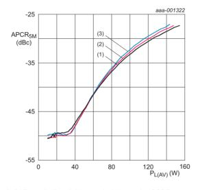
$V_{DS}$  = 28 V;  $I_{Dq}$  = 1900 mA; PAR = 7.2 dB at 0.01 % probability on the CCDF.
