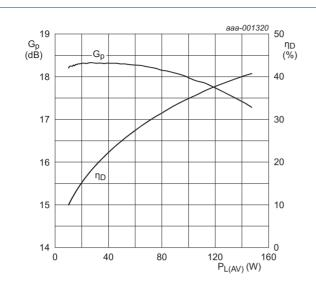
$V_{DS}$  = 28 V;  $I_{Dq}$  = 1900 mA; f = 2140 MHz; PAR = 7.2 dB at 0.01 % probability on the CCDF.
