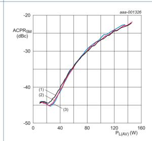
$V_{DS}$  = 28 V;  $I_{Dq}$  = 1900 mA; Channel Spacing = 5 MHz; PAR = 8.4 dB at 0.01 % probability on the CCDF.
