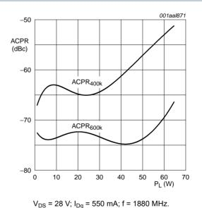
Fig 5. GSM EDGE ACPR at 400 kHz and at 600 kHz as function of load power; typical values
