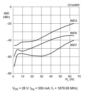
$f_2$  = 1880.05 MHz. Fig 3. Two-tone CW intermodulation distortion as a
