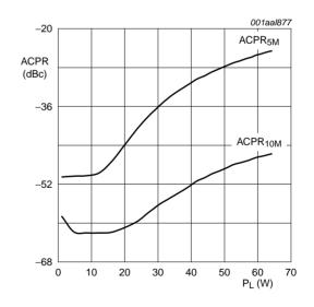
$V_{DS}$  = 28 V;  $I_{Dq}$  = 600 mA; f = 1880 MHz.
