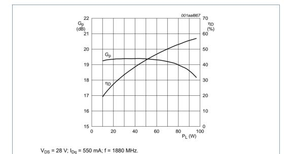
Fig 1. One-tone CW power gain and drain efficiency as function of load power; typical values
