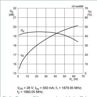
Fig 2. Two-tone CW power gain and drain efficiency as function of load power; typical values
