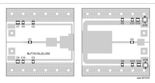
Printed-Circuit Board (PCB): Rogers RO3006;  $\varepsilon_r$  = 6.15 F/m; thickness = 0.635 mm; thickness copper plating = 35  $\mu$ m.
