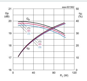
$V_{DS} = 30 \text{ V}; I_{Da} = 1800 \text{ mA}.$
