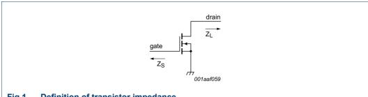
**Definition of transistor impedance**
