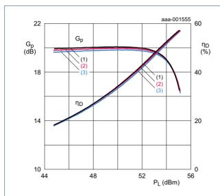
$V_{DS}$  = 30 V;  $I_{Dq}$  = 1800 mA.
