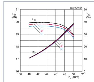
$V_{DS}$  = 30 V;  $I_{Dq}$  = 1800 mA.
