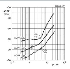
$V_{DS}$  = 28 V;  $I_{Dg}$  = 450 mA; f = 3500 MHz; Single Carrier N-CDMA; PAR = 9.7 dB at 0.01 % probability; Channel Bandwidth = 1.23 MHz; IBW = 30 kHz.
