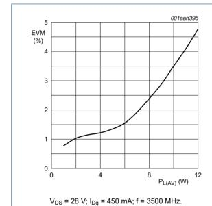
Fig 1. EVM as a function of average load power; typical values
