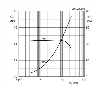
$V_{DS}$  = 28 V;  $I_{Dq}$  = 450 mA; f = 3500 MHz; Single Carrier N-CDMA; PAR = 9.7 dB at 0.01 % probability; Channel Bandwidth = 1.23 MHz; IBW = 30 kHz.
