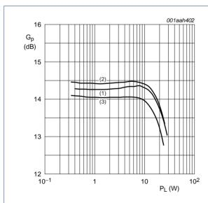
$V_{DS}$  = 28 V;  $I_{Dq}$  = 450 mA; Single Carrier N-CDMA; PAR = 9.7 dB at 0.01 % probability; Channel Bandwidth = 1.23 MHz; IBW = 30 kHz.
