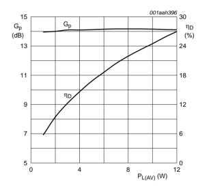
$V_{DS}$  = 28 V;  $I_{Dq}$  = 450 mA; f = 3500 MHz.
