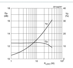
$V_{DS}$  = 28 V;  $I_{Dq}$  = 1050 mA; f = 3500 MHz; single carrier IS-95; PAR = 9.7 dB at 0.01 % probability; channel bandwidth = 1.23 MHz.
