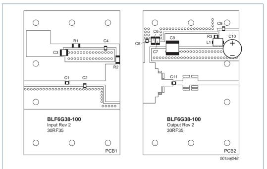
Striplines are on a double copper-clad Taconic RF35 Printed-Circuit Board (PCB) with  $\epsilon_{\text{r}}$  = 3.5 and thickness = 0.76 mm.
