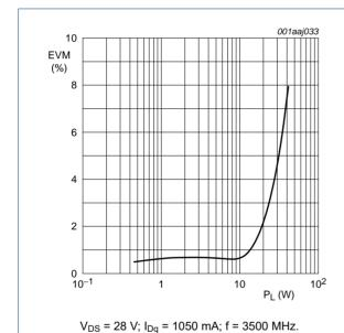
Fig 1. EVM as a function of load power; typical values
