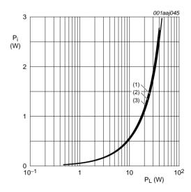
$V_{DS}$  = 28 V;  $I_{Dq}$  = 1050 mA; single carrier IS-95; PAR = 9.7 dB at 0.01 % probability; channel bandwidth = 1.23 MHz.
