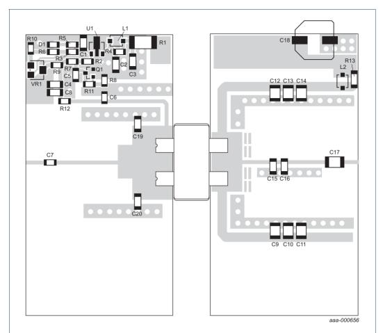
Printed-Circuit Board (PCB): Rogers RO4350;  $\epsilon_{\text{r}}$  = 3.5 F/m; thickness = 0.762 mm; thickness copper plating = 35  $\mu$ m.
