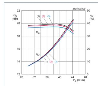
$V_{DS} = 28 \text{ V}; I_{Dq} = 410 \text{ mA}.$
