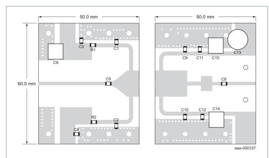
Printed-Circuit Board (PCB): Rogers RO4350;  $\epsilon_r$  = 3.5 F/m; thickness = 0.762 mm; thickness copper plating = 35  $\mu$ m.
