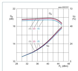
$V_{DS} = 28 \text{ V}; I_{Dq} = 410 \text{ mA}.$
