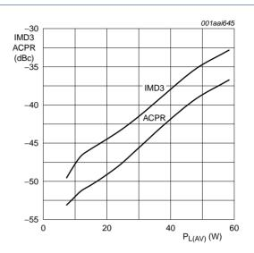
$V_{DS}$  = 30 V;  $I_{Dq}$  = 1400 mA; f = 2140 MHz (±5 MHz); carrier spacing 10 MHz.
