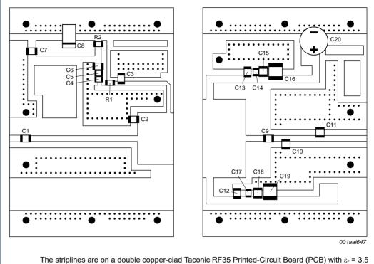
The striplines are on a double copper-clad Taconic RF35 Printed-Circuit Board (PCB) with  $\varepsilon_r$  = 3.5 and thickness = 0.76 mm.
