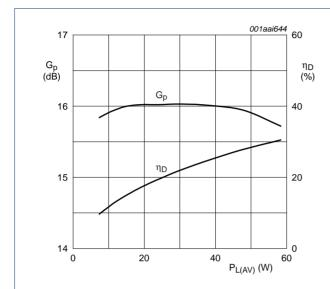
$V_{DS}$  = 30 V;  $I_{Dq}$  = 1400 mA; f = 2140 MHz ( $\pm 5$  MHz); carrier spacing 10 MHz.
