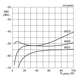
$V_{DS}$  = 30 V;  $I_{Dq}$  = 1400 mA; f = 2140 MHz.
