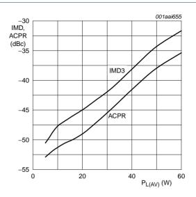
$V_{DS}$  = 30 V;  $I_{Dq}$  = 1400 mA; f = 1960 MHz (±5 MHz); carrier spacing 10 MHz.
