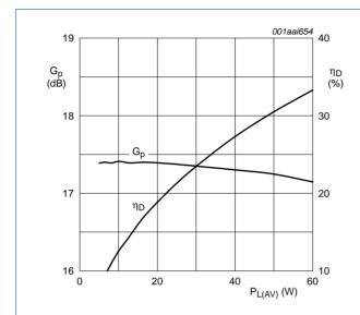
$V_{DS}$  = 30 V;  $I_{Dq}$  = 1400 mA; f = 1960 MHz ( $\pm 5$  MHz); carrier spacing 10 MHz.
