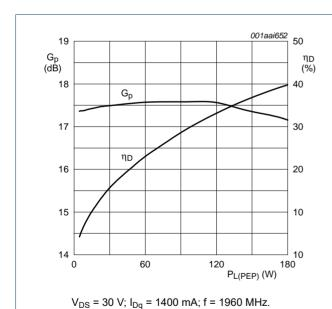
Fig 2. Two-tone CW power gain and drain efficiency as function of peak envelope load power; typical values
