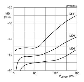
$V_{DS}$  = 30 V;  $I_{Dq}$  = 1400 mA; f = 1960 MHz.
