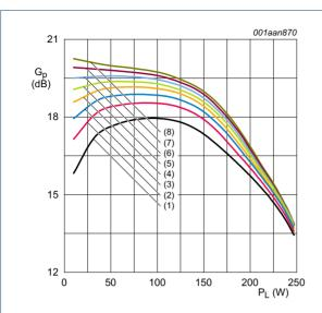
$V_{DS}$  = 50 V; f = 1300 MHz; carrier spacing = 100 kHz.
