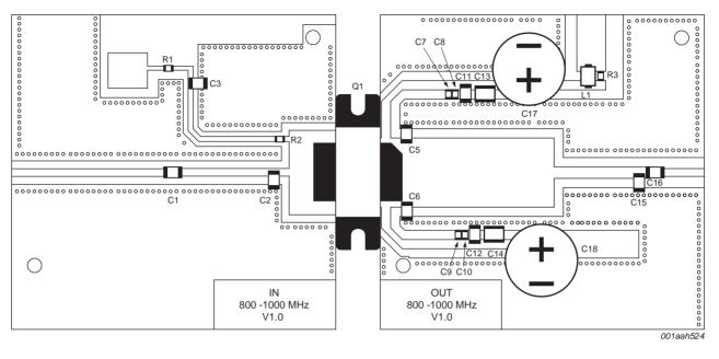
The striplines are on a double copper-clad Taconic RF35 Printed-Circuit Board (PCB) with  $\varepsilon_r$  = 3.5 and thickness = 0.76 mm. See <u>Table 8</u> for list of components.
