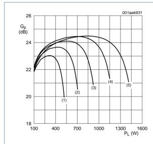
$I_{Dq}$  = 40 mA; f = 225 MHz;  $t_p$  = 100  $\mu$ s;  $\delta$  = 20 %.
