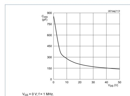
Fig 2. Output capacitance as a function of drain-source voltage; typical values per section
