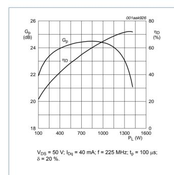
Fig 5. Power gain and drain efficiency as function of load power; typical values
