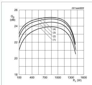
$V_{DS}$  = 50 V; f = 225 MHz;  $t_p$  = 100  $\mu$ s;  $\delta$  = 20 %.
