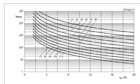
TTF (0.1 % failure fraction).
