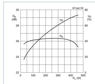
$V_{DS} = 50 \text{ V}$ ;  $I_{Dq} = 1000 \text{ mA}$ ; f = 225 MHz.
