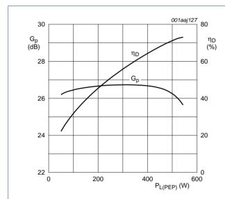
$V_{DS}$  = 50 V;  $I_{Dq}$  = 1000 mA; f = 225 MHz.
