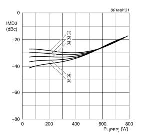
$V_{DS}$  = 50 V;  $f_1$  = 224.95 MHz;  $f_2$  = 225.05 MHz.
