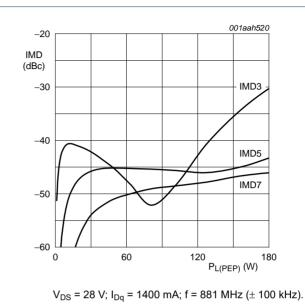
Fig 5. Intermodulation distortion as a function of peak envelope power load power; typical values
