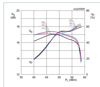
$V_{DS}$  = 32 V;  $I_{Dq}$  = 750 mA;  $V_{GS(amp)peak}$  = 1.18 V;  $t_p$  = 100  $\mu s; \, \delta$  = 10 %.
