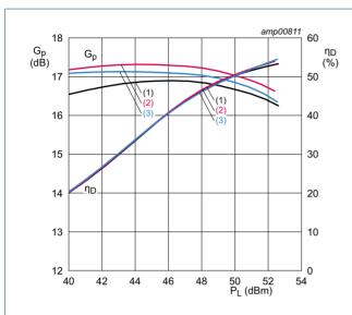
$V_{DS}$  = 32 V;  $I_{Dq}$  = 750 mA;  $V_{GS(amp)peak}$  = 1.18 V.
