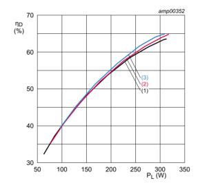
$V_{DS}$  = 32 V;  $I_{Dq}$  = 100 mA;  $t_p$  = 50  $\mu$ s;  $\delta$  = 2 %.
