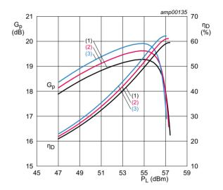
$V_{DS}$  = 50 V;  $I_{Dq}$  = 90 mA.
