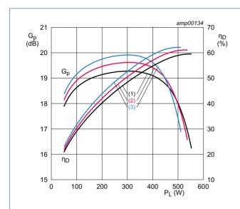
$V_{DS} = 50 \text{ V}; I_{Dq} = 90 \text{ mA}.$
