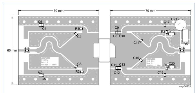
Printed-Circuit Board (PCB): Rogers RO4350;  $\epsilon_r$  = 3.48; height = 0.762 mm; thickness copper plating = 35  $\mu$ m. See Table 9 for a list of components.
