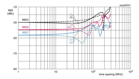
$T_{case} = 25 \, ^{\circ}\text{C}; \ V_{DS} = 28 \, \text{V}; \ I_{Dq(A\_P)} + I_{Dq(A\_C)} + I_{Dq(B\_P)} + I_{Dq(B\_C)} = 190 \, \text{mA} \, (carrier \, and \, peaking); \ V_{GS(A\_C)} = V_{GS(B\_C)} = 2.77 \, \text{V} \, (carrier); \ V_{GS(A\_P)} = V_{GS(B\_P)} = 1.65 \, \text{V} \, (peaking). \, \text{Test signal: 2-tone CW; } f_c = 1960 \, \text{MHz}.$
