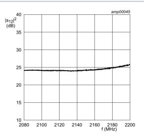
$T_{case}$  = 25 °C;  $V_{DS}$  = 28 V;  $I_{Dq}$  = 190 mA (carrier and peaking); measured on dual section evaluation board.
