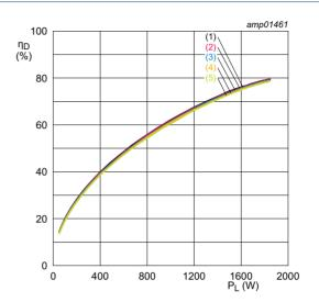
$V_{DS}$  = 55 V; f = 108 MHz;  $t_p$  = 100  $\mu s;$   $\delta$  = 10 %.
