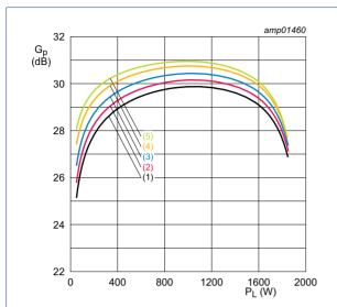
$V_{DS} = 55 \text{ V; } f = 108 \text{ MHz; } t_p = 100 \text{ } \mu\text{s; } \delta = 10 \text{ } \%.$
