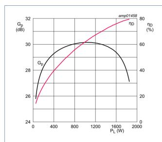
$V_{DS}$  = 55 V;  $I_{Dq}$  = 100 mA per section; f = 108 MHz;  $t_p$  = 100  $\mu s;~\delta$  = 10 %.
