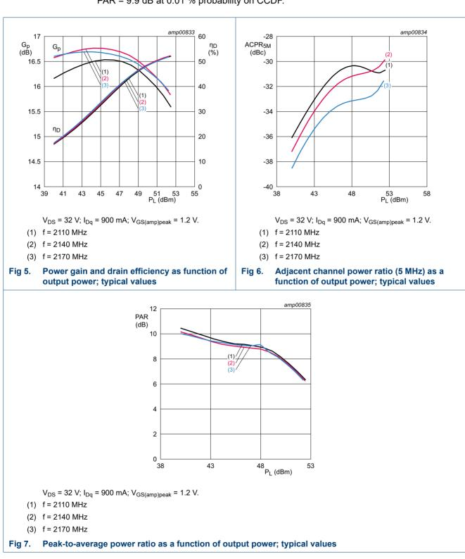
Test signal: 1-carrier W-CDMA; 3GPP test model 1; 1 to 64 DPCH (100 % clipping); PAR = 9.9 dB at 0.01 % probability on CCDF.
