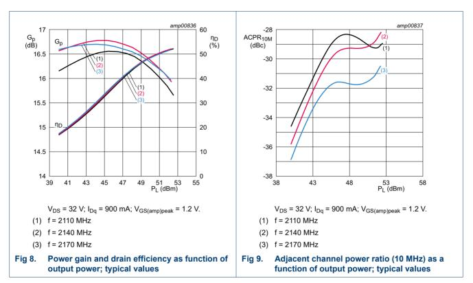
Test signal: 1-carrier LTE 10 MHz; PAR = 6.8 dB at 0.01 % probability on CCDF.
