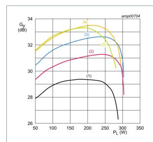
$I_{Dq1}$  = 25 mA;  $I_{Dq2}$  = 50 mA;  $V_{DS}$  = 32 V;  $T_{mb}$  = 25 °C.
