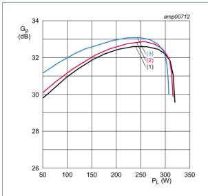
$I_{Dq1}$  = 25 mA;  $I_{Dq2}$  = 50 mA;  $V_{DS}$  = 32 V;  $T_{mb}$  = 25 °C; f = 2450 MHz.
