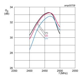
$I_{Dq1}$  = 25 mA;  $I_{Dq2}$  = 50 mA;  $T_{mb}$  = 25 °C.
