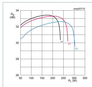
$I_{Dq1}$  = 25 mA;  $I_{Dq2}$  = 50 mA;  $T_{mb}$  = 25 °C; f = 2450 MHz.
