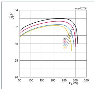
$I_{Dq1}$  = 25 mA;  $I_{Dq2}$  = 50 mA;  $V_{DS}$  = 32 V; f = 2450 MHz.
