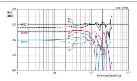
$T_{case}$  = 25 °C;  $V_{DS}$  = 28 V;  $I_{Dq1}$  = 30 mA;  $I_{Dq2}$  = 120 mA; f = 881 MHz; 2-tone CW;  $P_L$  = 8 W. Per section.
