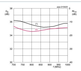
$T_{case}$  = 25 °C;  $V_{DS}$  = 28 V;  $I_{Dq1}$  = 30 mA;  $I_{Dq2}$  = 120 mA;  $P_{I}$  = 0.25 W. Per section.
