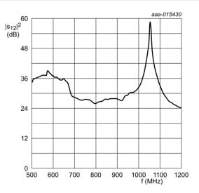
$T_{case}$  = 25 °C;  $V_{DS}$  = 28 V;  $I_{Dq1}$  = 30 mA;  $I_{Dq2}$  = 120 mA; measured on evaluation board.
