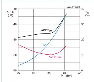
$T_{case}$  = 25 °C;  $V_{DS}$  = 28 V;  $I_{Dq1}$  = 30 mA;  $I_{Dq2}$  = 120 mA; f = 900 MHz; 1-carrier W-CDMA; test model 1; PAR = 9.9 dB at 0.01 % probability on CCDF. Per section.
