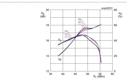
$V_{DS}$  = 32 V;  $I_{Dq}$  = 750 mA;  $V_{GS(amp)peak}$  = 1.18 V;  $t_p$  = 100  $\mu$ s;  $\delta$  = 10 %.
