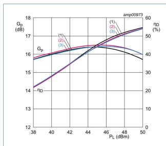
$V_{DS} = 32 \text{ V}; I_{Dq} = 750 \text{ mA}; V_{GS(amp)peak} = 1.18 \text{ V}.$
