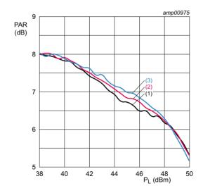
$V_{DS} = 32 \text{ V}; I_{Dq} = 750 \text{ mA}; V_{GS(amp)peak} = 1.18 \text{ V}.$
