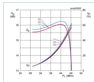
$V_{DS}$  = 50 V;  $I_{Dq}$  = 115 mA;  $t_p$  = 100  $\mu s; \, \delta$  = 10 %.
