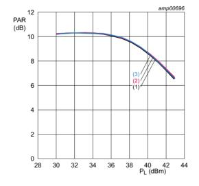
$V_{DS} = 50 \text{ V}; I_{Dq} = 115 \text{ mA}.$
