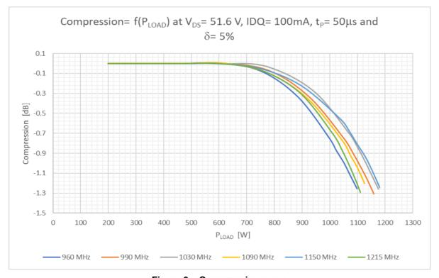
Figure 6 Compression curve
