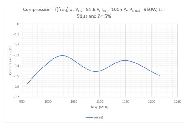
Figure 5 Compression at 950 W
