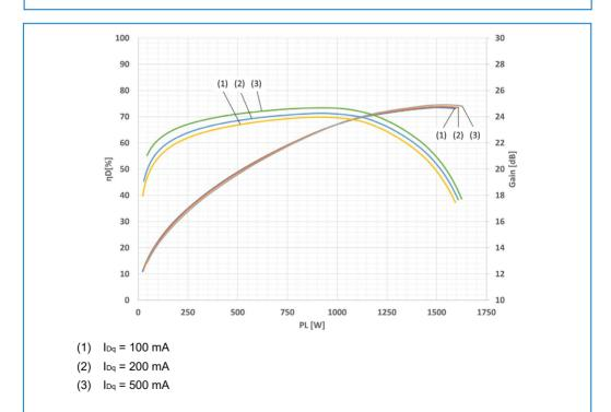
Fig 4. Gain and drain efficiency as function of output power; VDS = 65 V;  $\delta$  = 10 %
