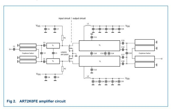
The demo board was built with double sided RT/duroid 6035HTC substrate material with  $\epsilon_r$  = 3.5. The substrate material has a height of 0.762 mm and the final copper thickness is 70 µm. Both input and output circuit use the same substrate material.
