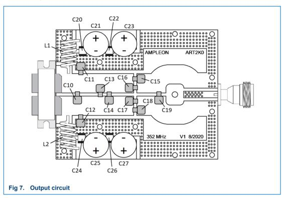
For demo purposes the output circuit makes use of a female N-connector for easy handling. It is however highly recommended to use a connector type that can handle higher power levels in a final application, like a 7/16 type connector.
