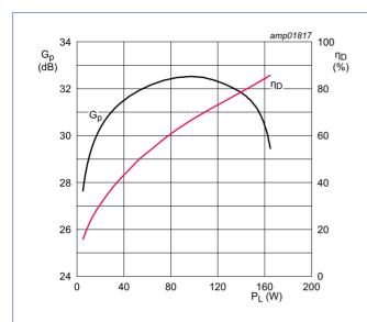
$V_{DS}$  = 65 V;  $I_{Dq}$  = 20 mA; f = 108 MHz;  $t_p$  = 100  $\mu s;$   $\delta$  = 10 %.
