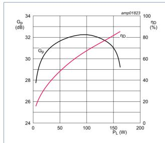
$V_{DS} = 65 \text{ V}; I_{Dq} = 20 \text{ mA}; f = 108 \text{ MHz}.$
