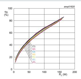
$V_{DS}$  = 65 V; f = 108 MHz;  $t_p$  = 100  $\mu$ s;  $\delta$  = 10 %.
