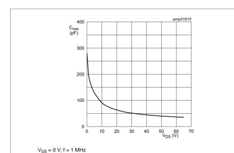
Output capacitance as a function of drain-source voltage; typical values Fig 2.
