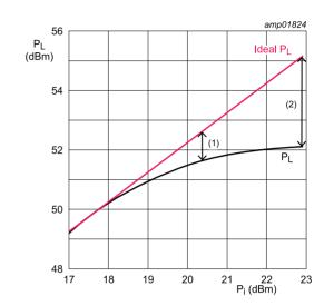
$V_{DS} = 65 \text{ V}; I_{Dq} = 20 \text{ mA}; f = 108 \text{ MHz}.$
