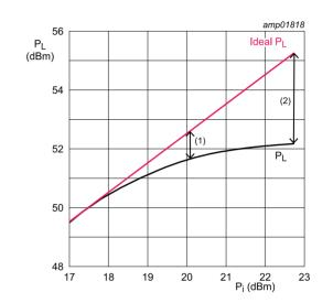
$V_{DS}$  = 65 V;  $I_{Dq}$  = 20 mA; f = 108 MHz;  $t_p$  = 100  $\mu s;$   $\delta$  = 10 %.
