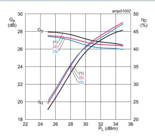
$V_{DS}$  = 28 V;  $V_{GS(amp)peak}$  =  $V_{GS(amp)main}$  - 0.55 V;  $I_{Dq}$  = 20 mA.
