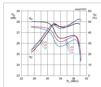
$$\begin{split} V_{DS} = 28 \text{ V; } V_{GS(amp)peak} = V_{GS(amp)main} - 0.55 \text{ V;} \\ I_{Dq} = 20 \text{ mA; } t_p = 100 \text{ } \mu\text{s; } \delta = 10 \text{ \%.} \end{split}$$
