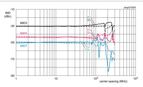
$V_{DS}$  = 28 V;  $V_{GS(amp)peak}$  =  $V_{GS(amp)main}$  – 0.55 V;  $I_{Dq}$  = 20 mA; f = 2600 MHz.
