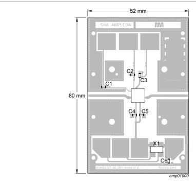
Printed-Circuit Board (PCB): Rogers 4350B;  $\epsilon_{\text{r}}$  = 3.66; thickness = 0.508 mm; thickness of copper plating = 35  $\mu$ m.
