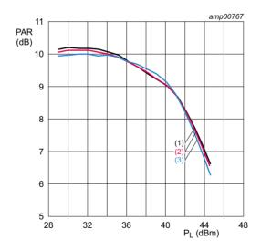
$V_{DS}$  = 28 V;  $I_{Dq}$  = 200 mA;  $V_{GS(amp)peak}$  = 0.6 V.
