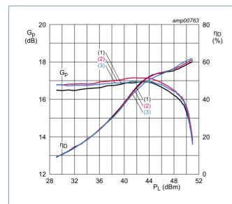
$V_{DS}$  = 28 V;  $I_{Dq}$  = 200 mA;  $V_{GS(amp)peak}$  = 0.6 V.
