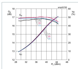
$V_{DS}$  = 28 V;  $I_{Dq}$  = 200 mA;  $V_{GS(amp)peak}$  = 0.6 V.
