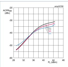
$V_{DS}$  = 28 V;  $I_{Dq}$  = 200 mA;  $V_{GS(amp)peak}$  = 0.6 V.
