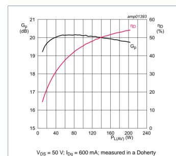
production test circuit at 550 MHz.
