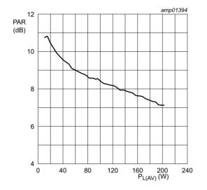
$V_{DS}$  = 50 V;  $I_{Dq}$  = 600 mA; measured in a Doherty production test circuit at 550 MHz.
