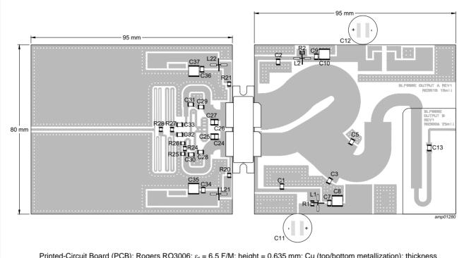
Printed-Circuit Board (PCB): Rogers RO3006;  $\epsilon_r$  = 6.5 F/M; height = 0.635 mm; Cu (top/bottom metallization); thickness copper plating = 29.6  $\mu$ m; Rogers RO3010;  $\epsilon_r$  = 10 F/M; height = 0.254 mm.
