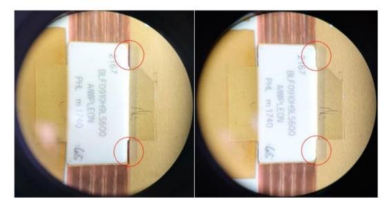
Figure 3. The gap between drain and PCB should be minimized
