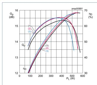
$V_{DS} = 32 \text{ V}; I_{Dq} = 20 \text{ mA}.$
