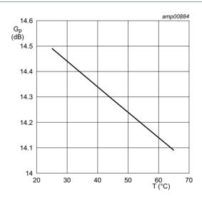
$V_{DS}$  = 32 V;  $I_{Dq}$  = 20 mA: f = 2450 MHz; at  $P_{L(1dB)}$ .
