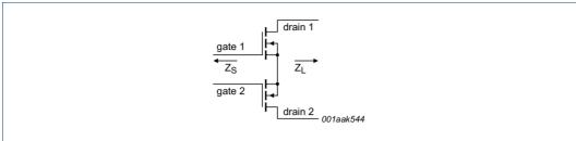
Fig 1. Definition of transistor impedance
