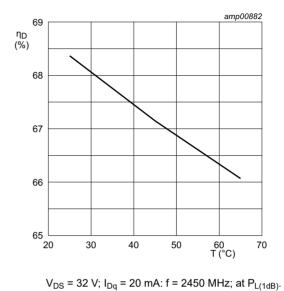
Fig 4. Drain efficiency as a function of temperature;
