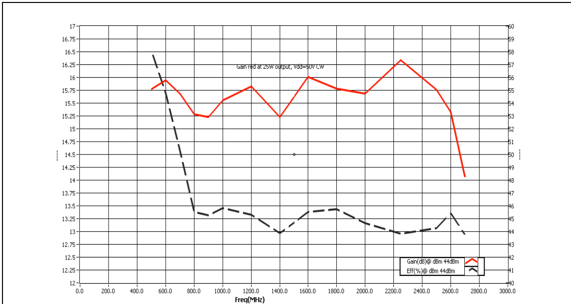
Figure 6. Gain(dB), Eff(%) vs Frequency(MHz)
