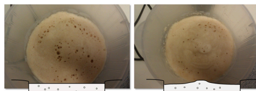
A thick pancake batter demo load heated first using all frequencies evenly, and secondly with an adaptive heating algorithm biased to use only the best modes for efficient cavity power retention
