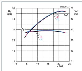
$V_{DS} = 32 \text{ V}$ ;  $I_{Dq1} = 10 \text{ mA}$ ;  $I_{Dq2} = 20 \text{ mA}$ ; CW test signal.
