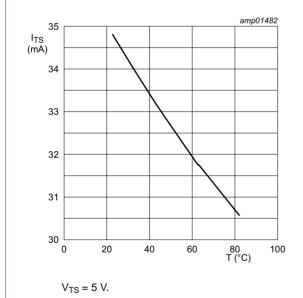
Fig 7. Temperature sensor current as a function of temperature; typical values
