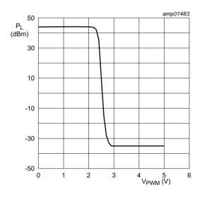
$V_{DS}=32$  V;  $P_i=15$  dBm; f = 2450 MHz;  $I_{Dq1}=10$  mA;  $I_{Dq2}=20$  mA;  $T_{water}=25\ ^{\circ}C$  (at water-cooled heatsink).
