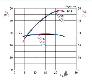
$V_{DS}$  = 32 V;  $I_{Dq1}$  = 10 mA;  $I_{Dq2}$  = 20 mA; CW pulsed test signal:  $t_p$  = 100  $\mu s;~\delta$  = 10 % .
