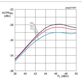
$V_{DS} = 30 \text{ V}; I_{Dq} = 300 \text{ mA}; V_{GS(amp)peak} = 1.3 \text{ V}.$
